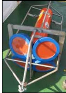
**Plate 4.** Upward looking ADCP on the LOCO moorings
