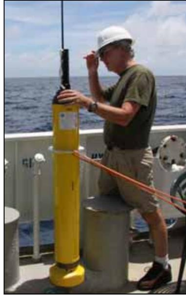
**Plate 2.** Argo float ready for deployment
