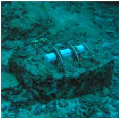
**Plate 5.** Underwater Temperature Recorder
